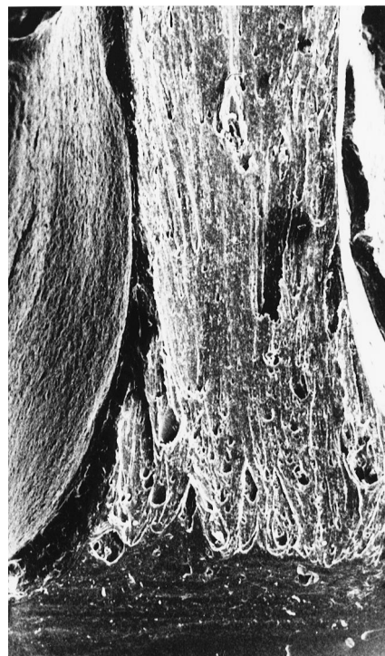
Figure 13 Fracture surface of the PA/PSU 251 (68/32) at low magnification
